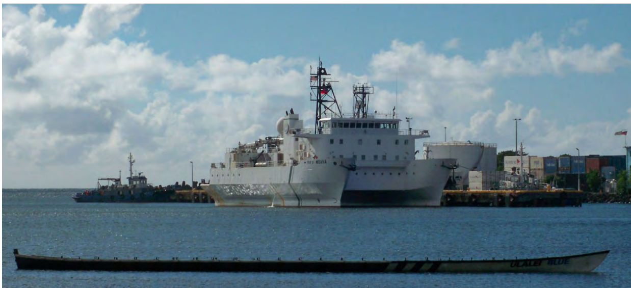
Figure 1.1: The R/V Kilo Moana in Apia, Western Samoa, in 2010. The Kilo Moana is a SWATH (Small Waterplane Area Twin Hull) vessel owned by the U.S. Navy and operated by the University of Hawai'i.
