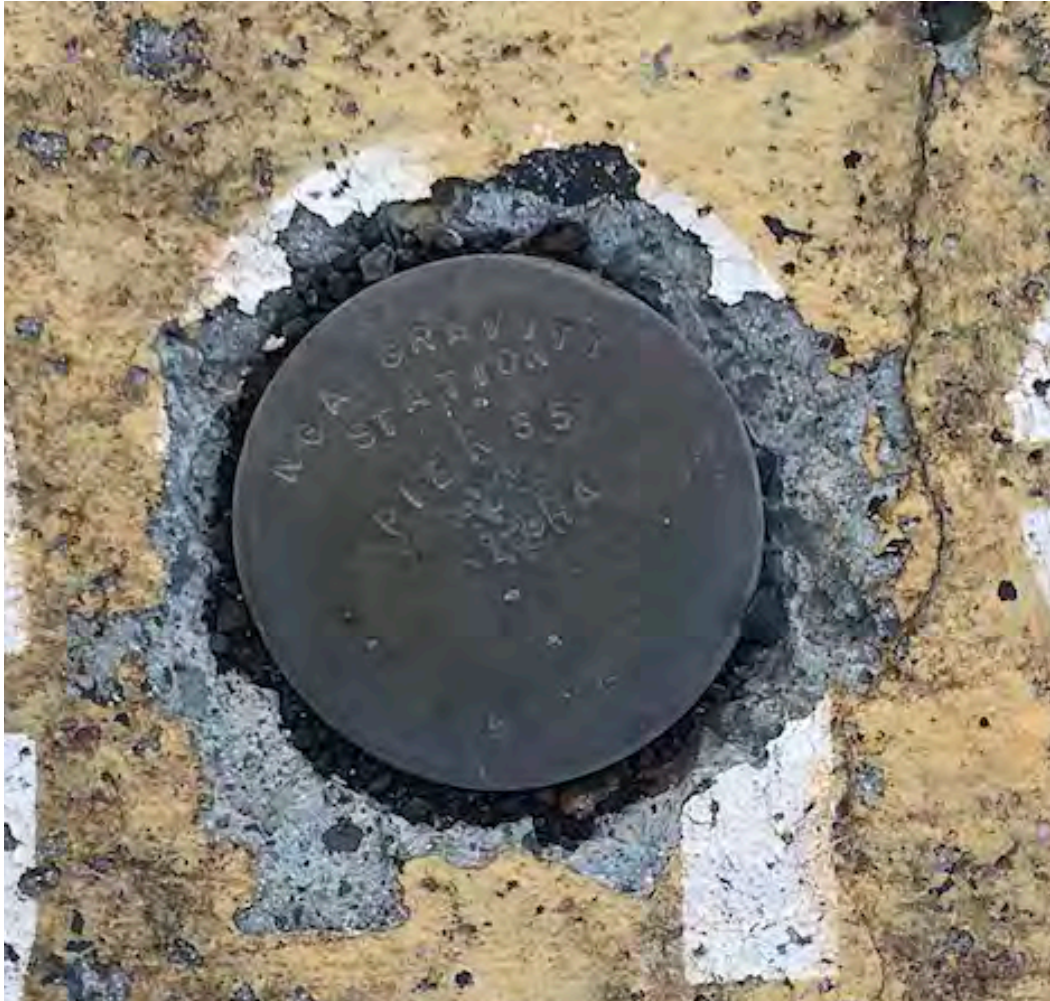
Figure D.7: Gravity station monument corresponding to the station description in Figure D.6.
