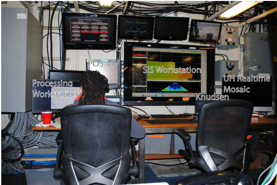
Figure 2.1: Instrument displays in the main lab of the KiloMoana during KM17-18. The large center screen is used for SIS, and the screen to the left displays the POS/MV real-time performance metrics, while the laptop to the right was used for Knudsen display. The laptop to the left was used for data processing and quality control. A separate real-time data mosaic service was provided by University of Hawai'i (far right) but was not used for survey purposes.
