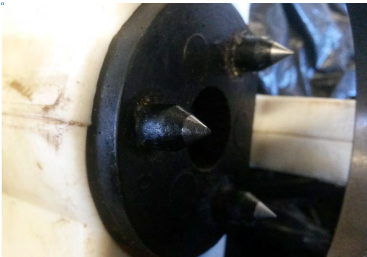
Figure 13: Detail of the XBT launcher with the corroded terminal connector (left). Intermittent contact with the pads in the XBTs caused failures in recognizing new probes, and in collecting data during operations. A new launcher was subsequently substituted.
