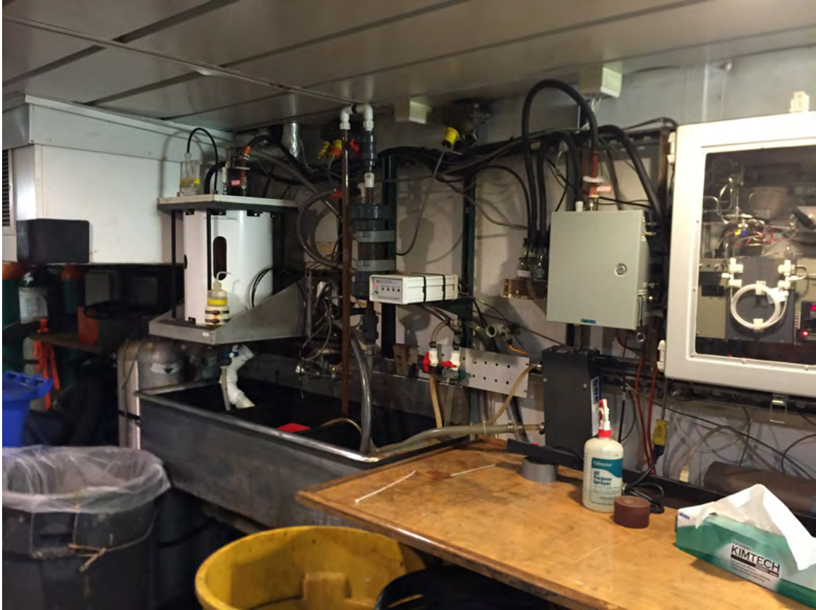
Figure 6: The main-deck wet lab of the R/V Langseth during MGL15-12. The de-bubbler for the TSG is the wall-mounted grey cylinder in the center of the image, with the white pCO 2 tank to the left, and the gas analyzer to the far right. The dark grey box plumbed into the sink is the TSG.
