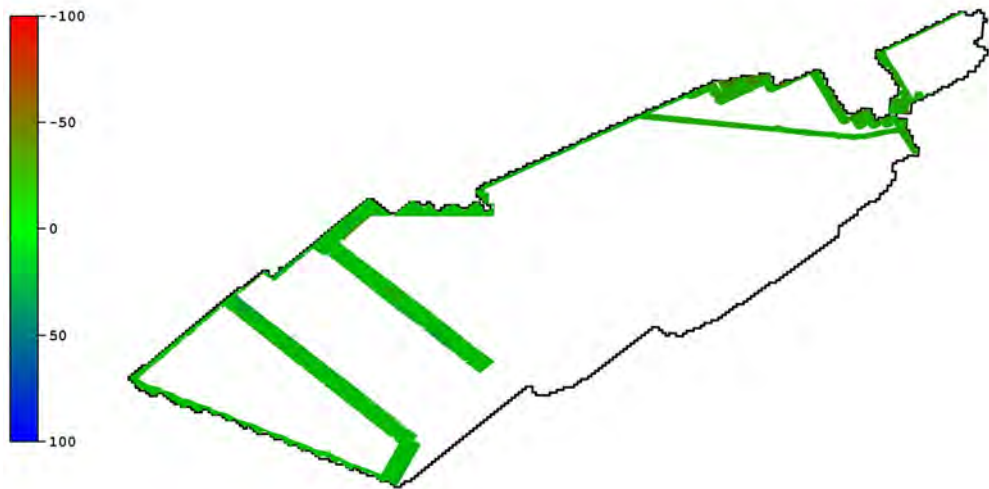
Figure 23: Surface differences between previous legs of the U.S. east coast mapping campaign, Okeanos Explorer EX13-03, and leg 8 (black outline). Differences range between -215m and 274m, with mean -0.8m and standard deviation 11.6m.
